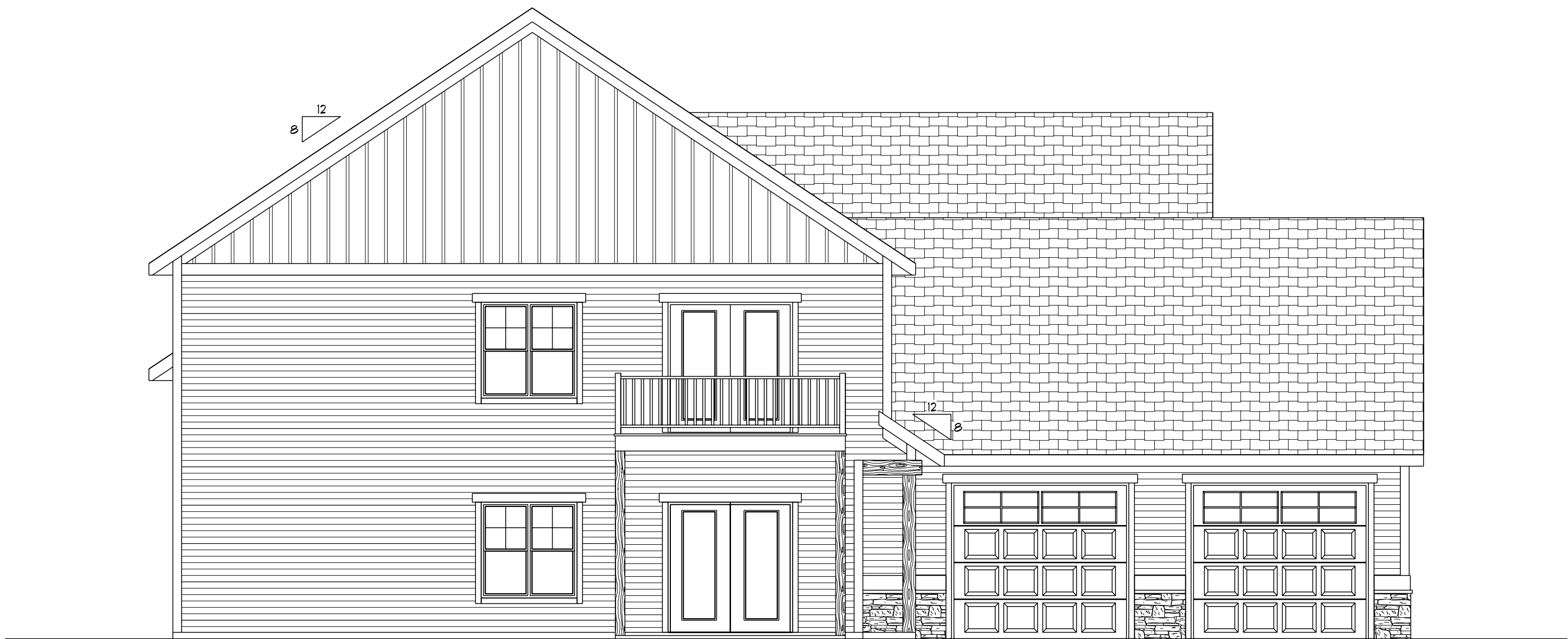
LEFT ELEVATION SCALE: 3/16" = 1'-0"
