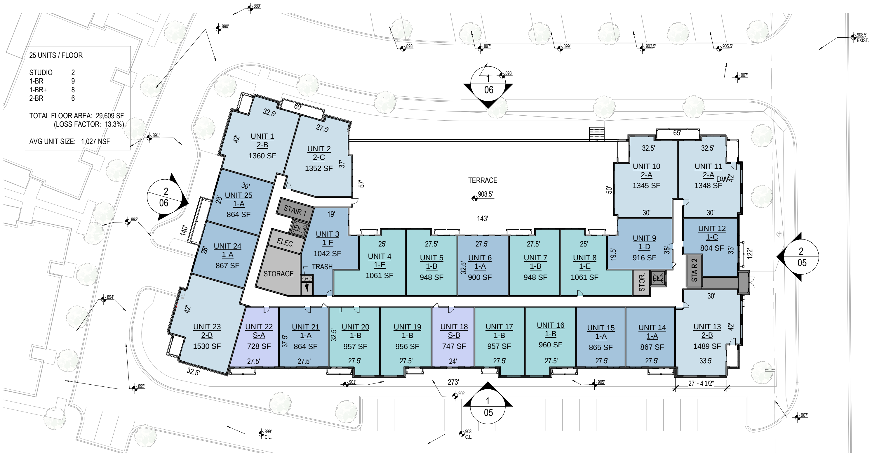
1 FIRST FLOOR PLAN SCALE: 1" = 30'-0"
