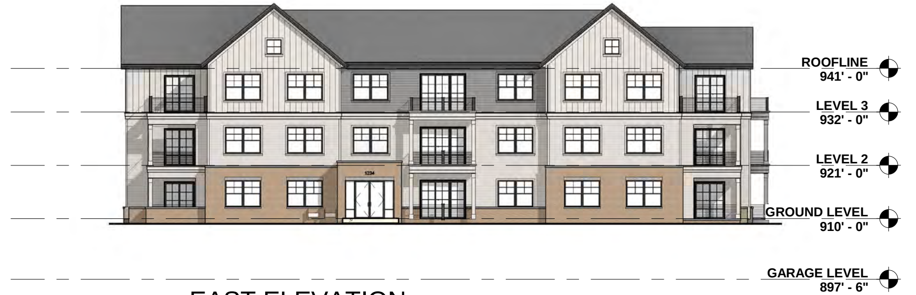
2 EAST ELEVATION SCALE: 1" = 20'-0"
